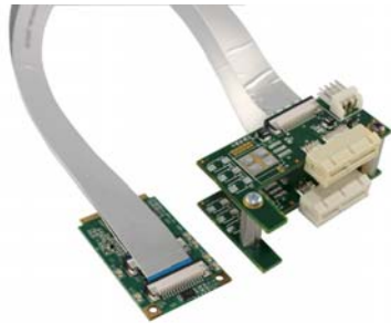
Figure 1: Flexible MiniPCIe to 2x PCIe Splitter
