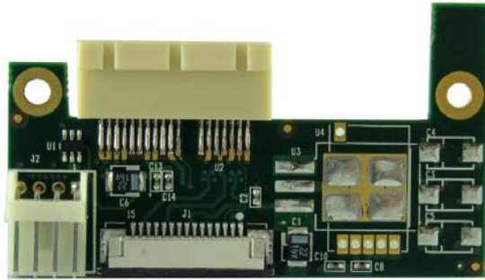
Figure 3: x1 PCI Express adapter board (powered from host card (3.3V only))
