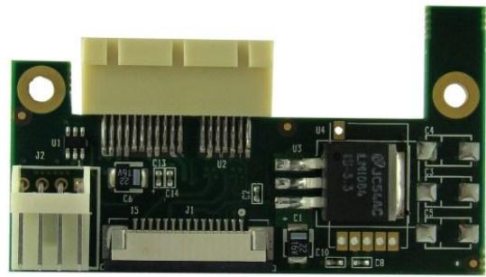
Figure 4: x1 PCI Express adapter board (powered from ATX power supply) (12V, 5V)
