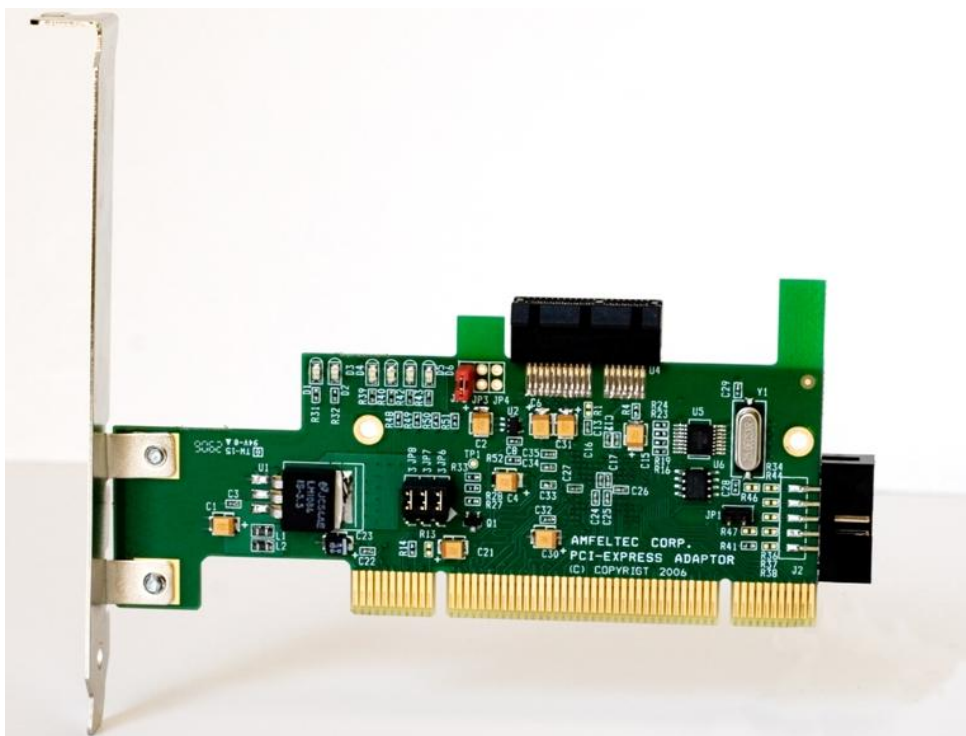
Figure 1: PCI to PCI Express Adapter
