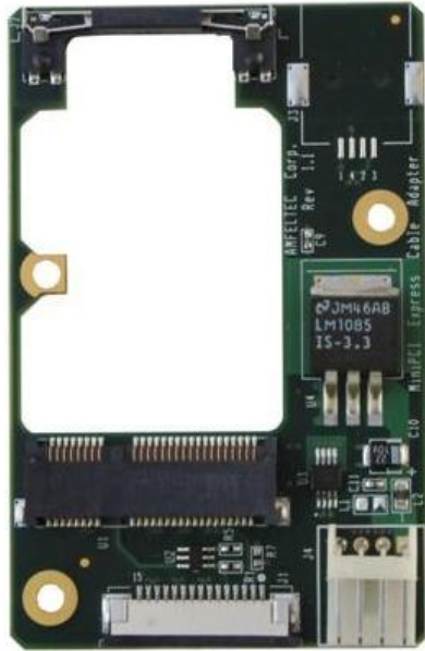
Figure 3: MiniPCI Express Adapter board
