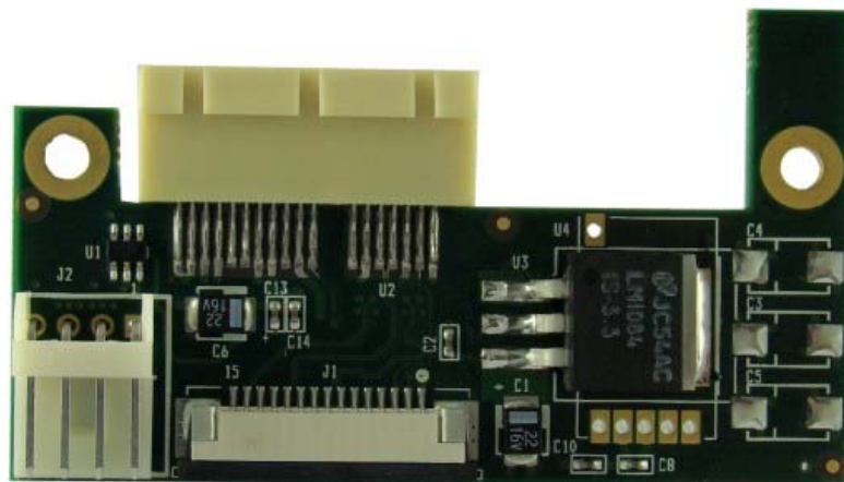
Figure 5: x1 PCI Express adapter board (powered from ATX power supply) (12V, 5V)
