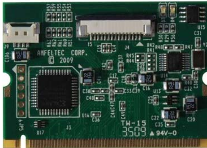
Figure 2: MiniPCI Host Card
