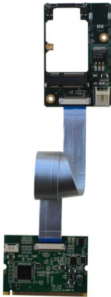
Figure 1: Flexible MiniPCI to MiniPCI Express Adapter
