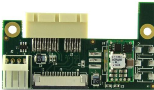
Figure 5: x1 PCI Express adapter board (powered from external 12V power supply)
