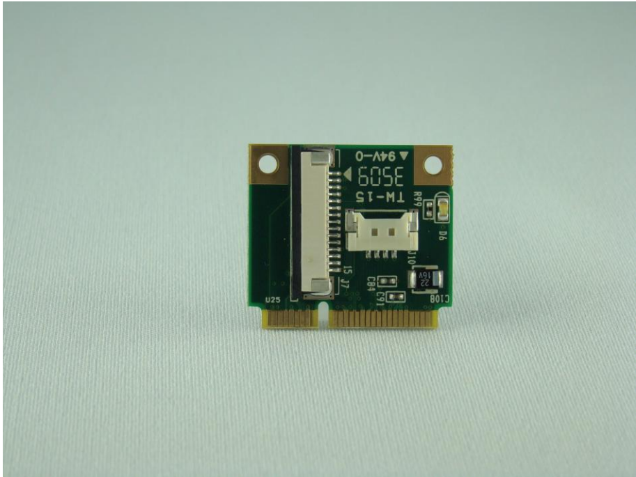
Figure 2b: MiniPCI Express Host board (half size)
