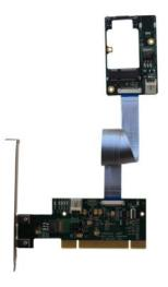
Figure 1: Flexible PCI to MiniPCIe Adapter
