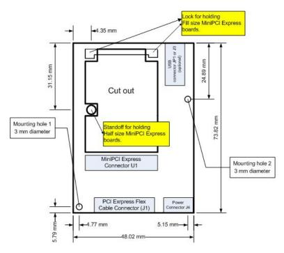
Figure 5: MiniPCI Express Adapter board layout
