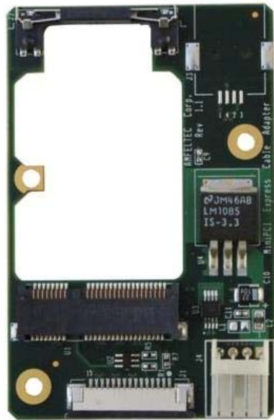
Figure 3: MiniPCI Express Adapter board.
