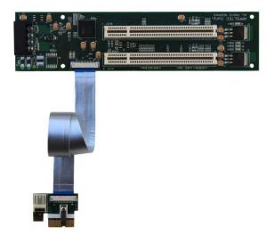
Figure 1: Flexible x1 PCIe to PCI Bus Adapter
