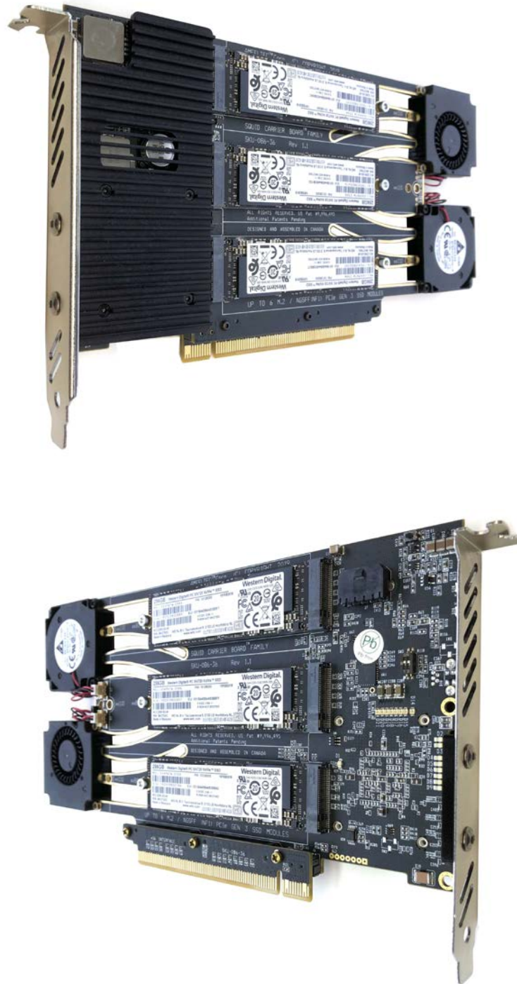
Figure 1: PCIe Gen 3 Carrier Board with six M.2 SSD modules (top and bottom sides)
