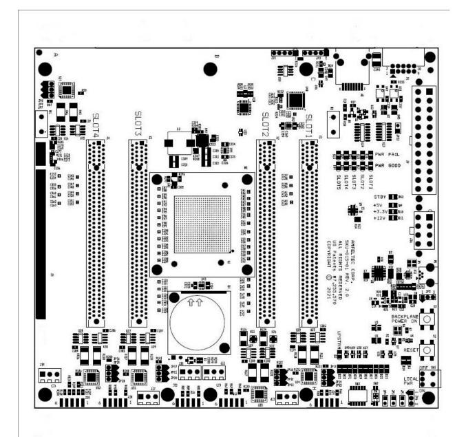
Figure 6: PCI Express Gen 3 Test Backplane component placement
