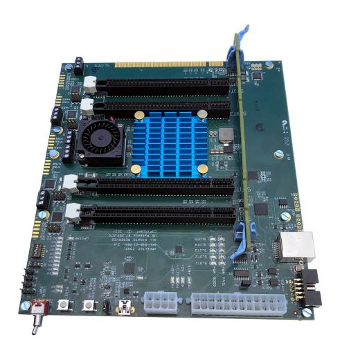
Figure 1: PCI Express Gen 3 Test Backplane
