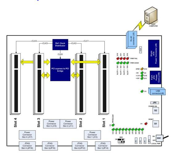
Figure 5: PCI Express Gen 3 Test Backplane block diagram
