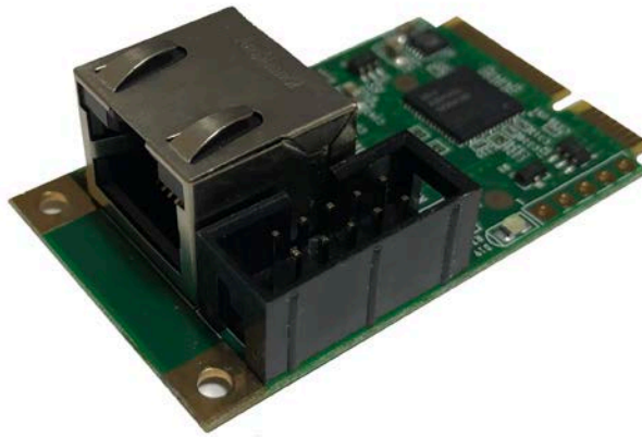
Figure 4: MiniPCI Express Host board
