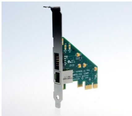
Figure 2: PCI express Host board
