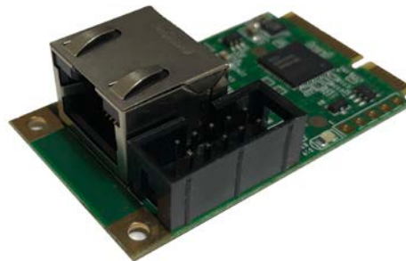
Figure 3: MiniPCI express Host board
