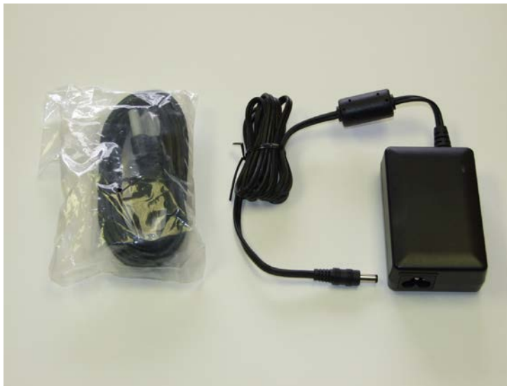
Power supply for MiniPCI Express Backplane.
