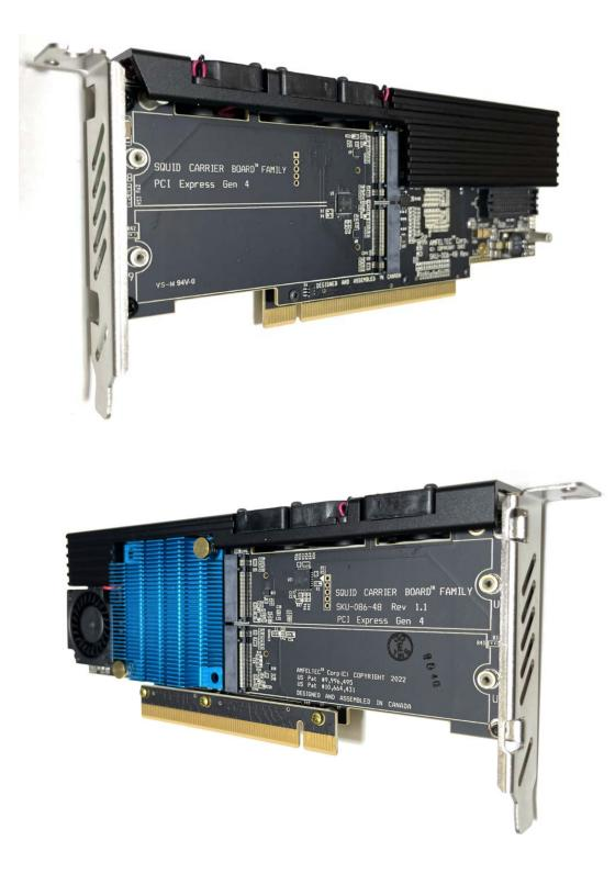
Figure 1: PCIe Gen 4.0 Carrier Board with four M.2 SSD modules (top and bottom sides)
